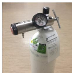
**In either case the connecting mount to the flow meter should be checked for leaks. Usually a leak is audible on careful listening**
